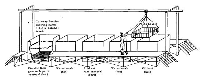
Figure 33. Central degreasing and paint removal system.
