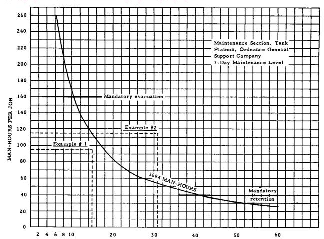
Figure 32. Variable repair time limits.
