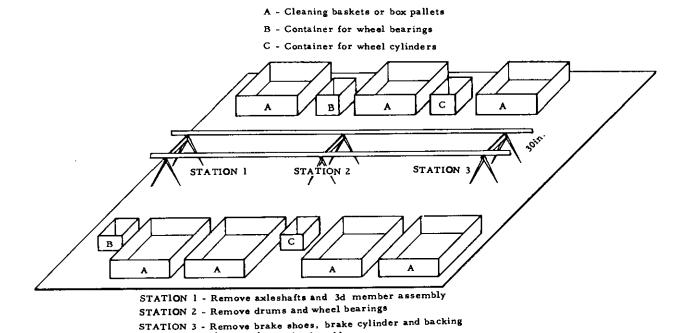
Figure 39. Axle disassembly area.
