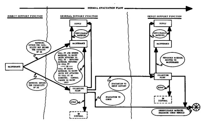
Figure 4. Ordnance evacuation flow, class II and IV (less guided missiles).
